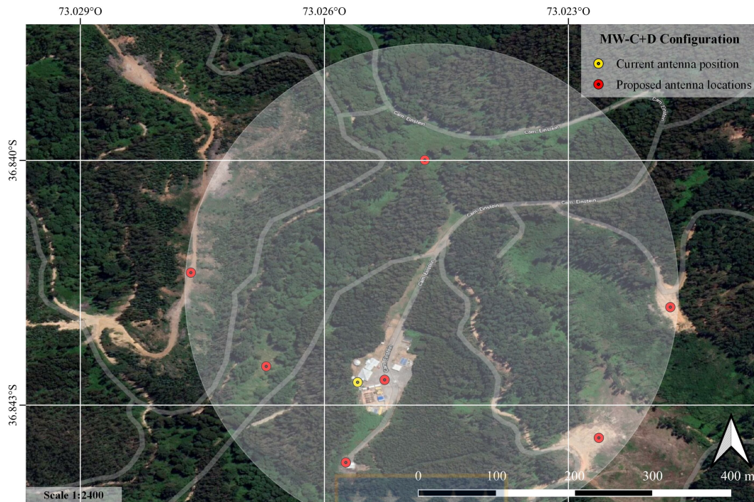
Figure 4.2.8: Antenna position for the MW-C+D array configurations. White circle has a radii of 509 meters which corresponds to the maximum antenna separation distance. Maps generated with the Quantum Geographic Information System (QGIS version 3.16.13) using Google Maps Hybrid as layer map. White arrow points North and antenna symbols are not to scale.
