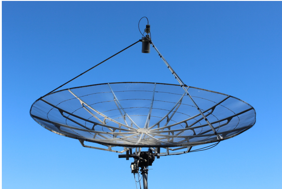
Figure 1.1.1: 3 meters mesh-parabolic dish antenna in the WenuLafquen observatory at the University of Concepcion. Notice the 12 arms acting as "ribs" and the feed horn antenna. Image from the note Panorama Udec
