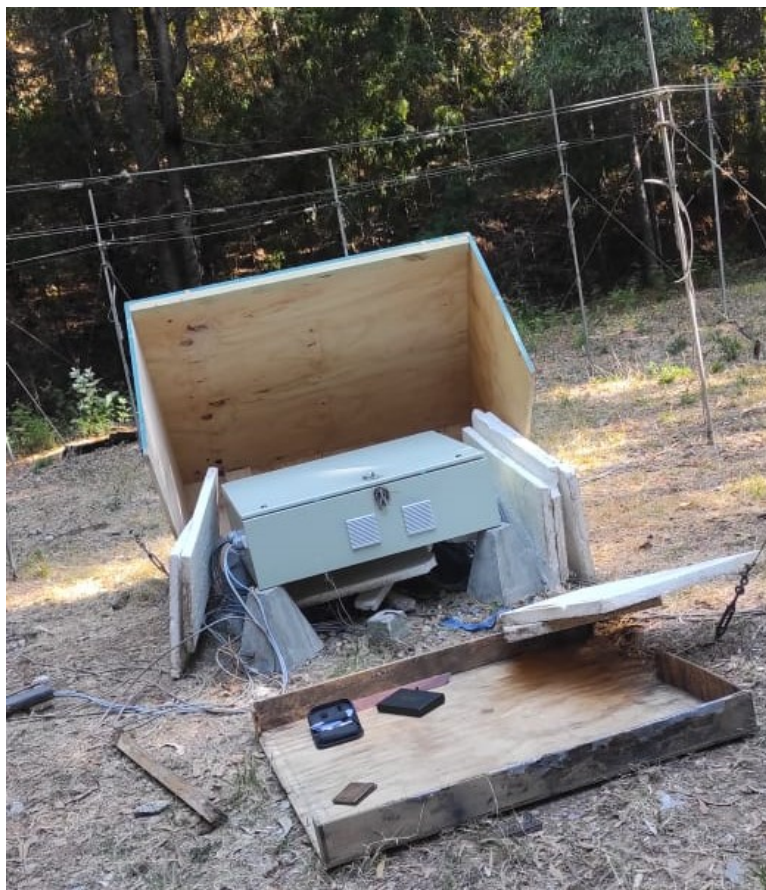
Figure 3.5.8: Picture of the metal box for hardware of ISI-RIOmeter and external wood box to reduce the heating by sun radiation. .
