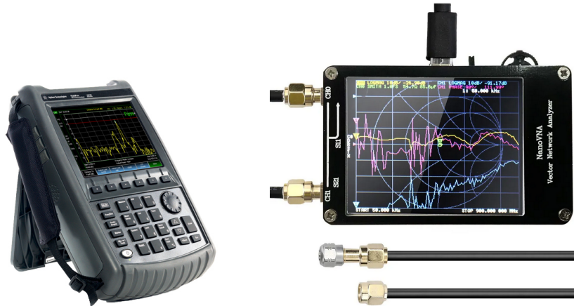
Figure 3.2.4: On the right the vector network analyzer model N9918A and on the left the NanoVNA
