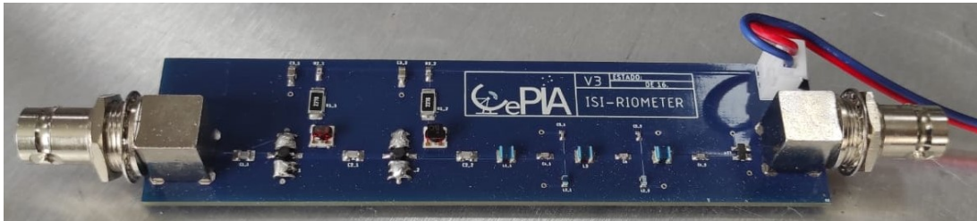
Figure 3.3.12: Photograph of the final assembled PCB, Dimensions 120 x 30 [mm]
