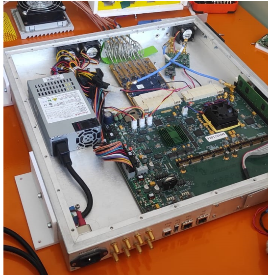
Figure 3.4.5: ROACH2, ADC16x250-8 and valon 5007.
