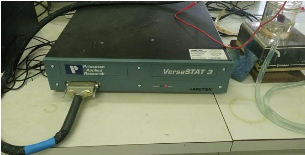
Figura 22: Potenciostato VersaStat 3.
