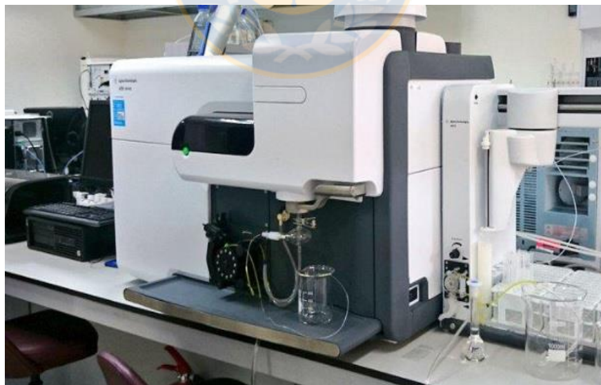
Figure 10. Agilent 4200 MP-AES microwave plasma-atomic emission spectrometer used to analyze liquid samples.
