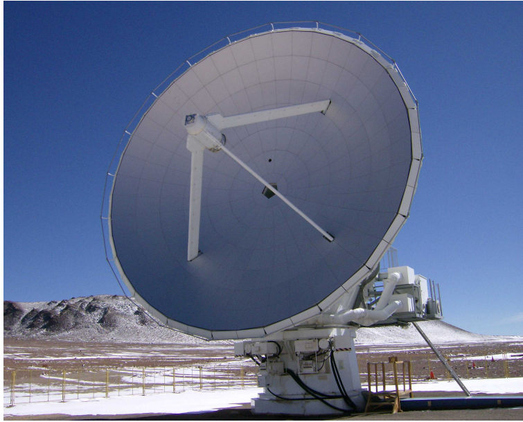
Figure 3.2: ASTE is located 4,800 meters above sea level, at the Atacama Desert in Northern Chile, it observes sub-millimeter ( 0.1[mm]-1[mm] ) wavelengths. Telescope diameter is 10[m] and Beam size at 350 [GHz] is 22'' .
