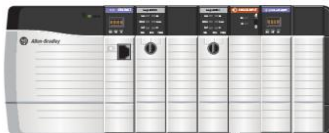
Fig. C.1. PLC Control Logix
