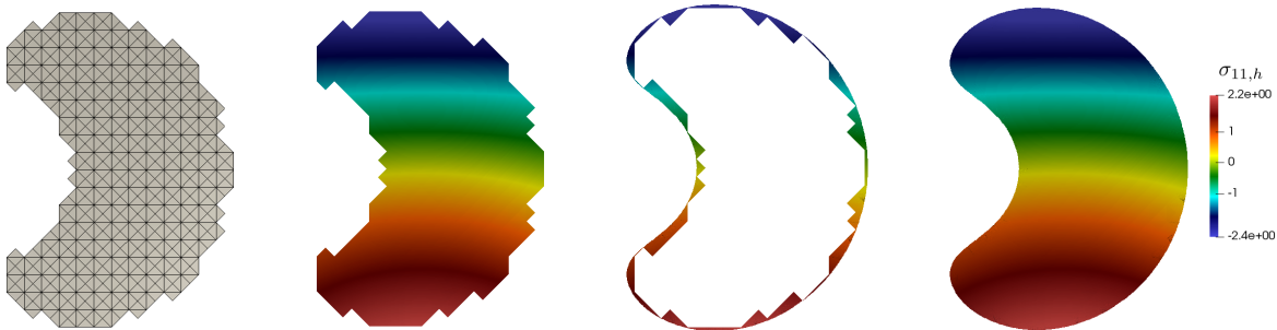
Figure 2.4: Example 1: Approximate pseudostress component \sigma_{11,h} obtained with N = 654 and k = 2 . (figure produced by the author)
