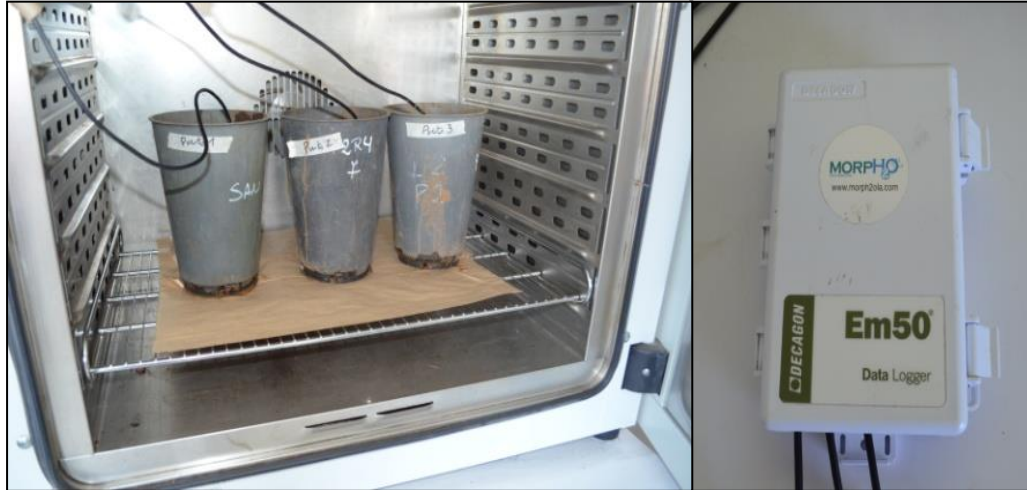
Figure S1. Pots inside oven used for calibrating the sensors used to record variations in volumetric moisture content during the calibration period.
